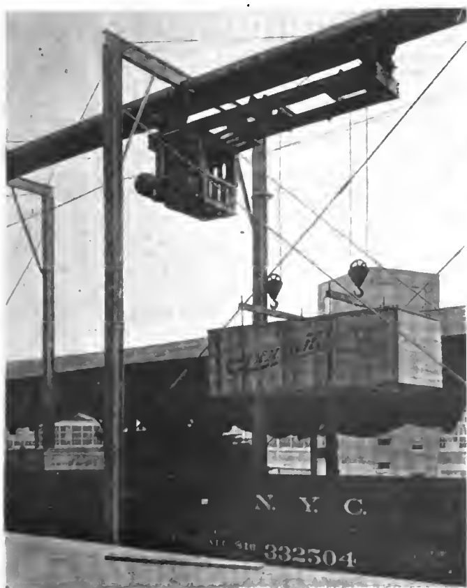
Below the new electric crane at the plant of the Willys-Overland Co., Toledo, is illustrated picking up a box containing an automobile packed for export shipment preparatory to moving it to the waiting freight car
